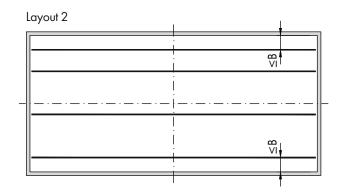
The fixing points of the hangers are determined by the layout of the Main Runners. The distance of the first and last Main Runner from the wall should be smaller than module width B, so that laying long Cross Tees on the perimeter trim is avoided.
